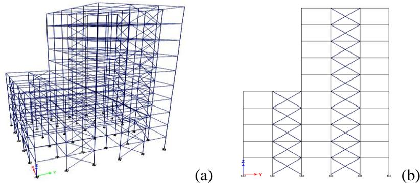
**Figure 3.** Model for plan and elevation irregular concentrically braced steel frame with a setback of five top stories: (a) 3D; and (b) plane frame
