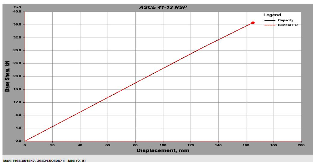
**Figure 10.** Capacity curve and bilinear idealization of inclined frame model of concentrically braced steel frame
