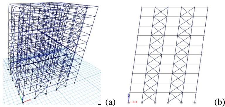
**Figure 5.** Model for inclined concentrically braced steel frame: (a) 3D; and (b) plane frame
