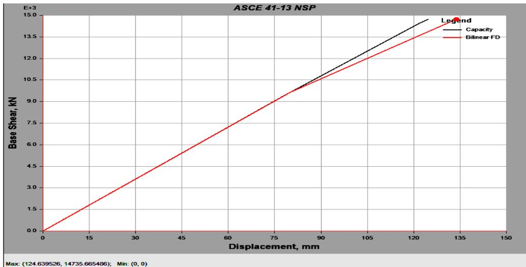
**Figure 8.** Capacity curve and bilinear idealization of plan and elevation irregular concentrically braced steel frame with a setback of five top stories
