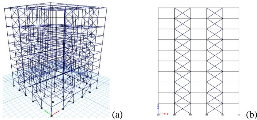
**Figure 1.** Model for regular in plan and elevation concentrically braced steel frame: (a) 3D; and (b) plane frame
