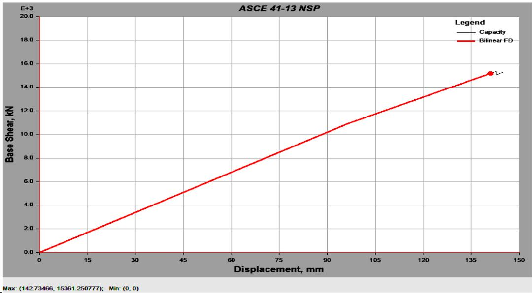
**Figure 6.** Capacity curve and bilinear idealization of plan regular frame model of plan regular concentrically braced steel frame
