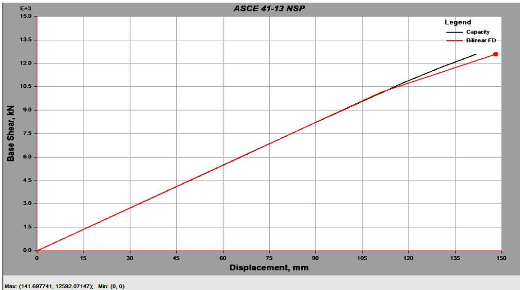
**Figure 7.** Capacity curve and bilinear idealization of plan irregular frame model of concentrically braced steel frame
