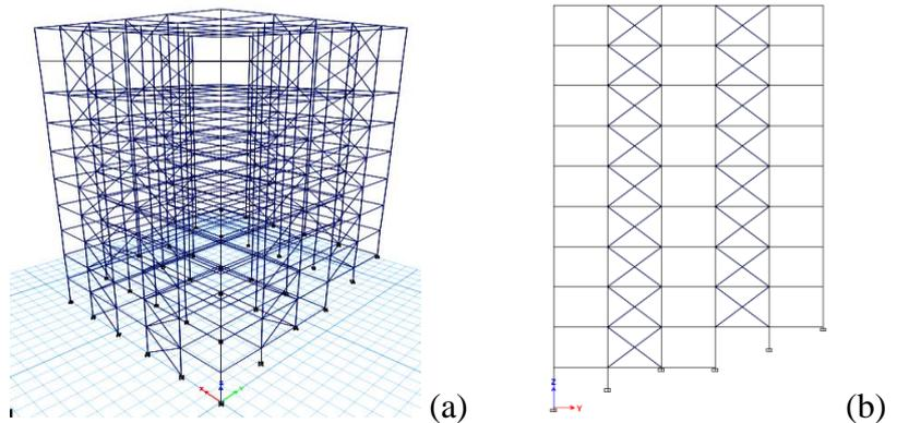
**Figure 4.** Model for concentrically braced steel frame with setback of two bottom stories in the y direction: (a) 3D; and (b) plane frame
