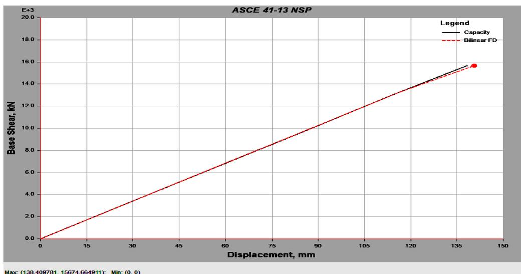
**Figure 9.** Capacity curve and bilinear idealization of down setback frame model of concentrically braced steel frame with setback of two bottom stories in the y direction
