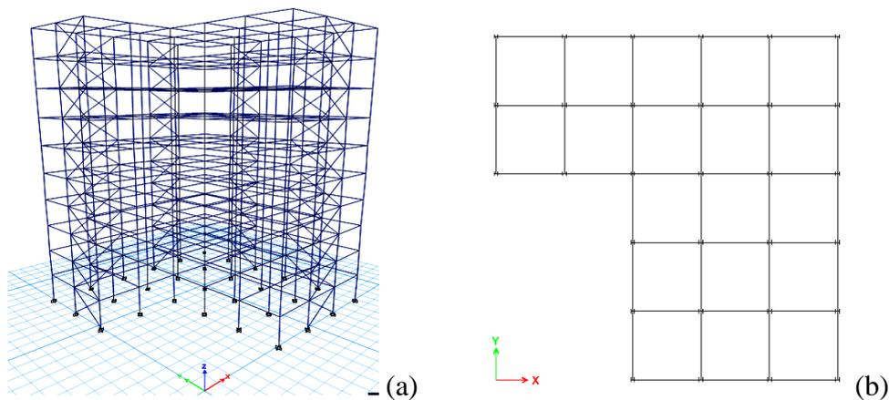
**Figure 2.** Model for plan irregular concentrically braced steel frame: (a) 3D; and (b) floor plan
